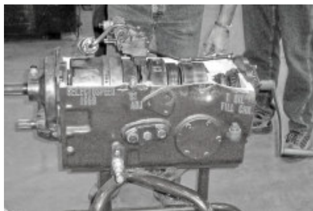
Cut away of Ford Select-O-Speed transmission with hand crank (at right) to demonstrate operation.
